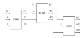
Fig. 5 (a) 2x4 Decoder using 3 FDK gates
