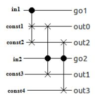
Fig 5(b) Circuit of Reversible Decoder using FDKs
