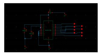
Fig. 10 Test circuit for 2x4 Decoder using 1FEYNMAN & 2FDK gates
