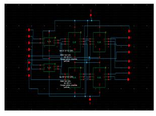
Fig 8. 2x4 Decoder using 2FEYNMAN & 4 TOFFOLI gates
