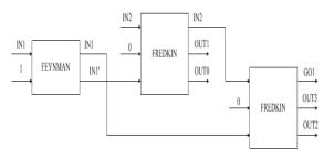
Fig. 6 2x4 Decoder using 1FEYNMAN & 2FDK gates
