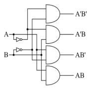
Fig1 (b) schematic / gate level of 2x4 Decoder circuit.
