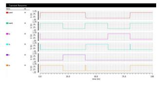
Fig 11 Output waveforms of 2x4 Decoder
